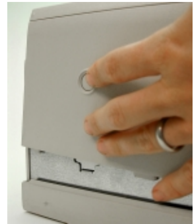
This Dell computer cover is opened by simply pushing two buttons on either side of the cover. No tool is required and the connectors are integral to their corresponding parts.
